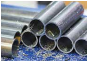
Burr ends of cut metal tubing
