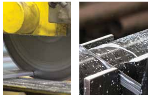
Examples of how metal tubing is cut
