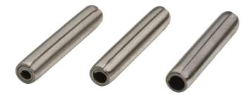
The **duty** (or material) thickness of the coiled pin can be varied to provide the optimum combination of strength and flexibility. The lighter duty pins require less insertion force, thus reduces the cost of the automation equipment
