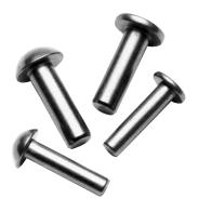
In order to utilize traditional automating methods, headed parts should be able to hang by the head. A good rule of thumb is that there should be a minimum of a 20% differential between the head and body diameter in order to provide enough distinction to allow for orienting and hanging the parts. If the diameter differential can be held
